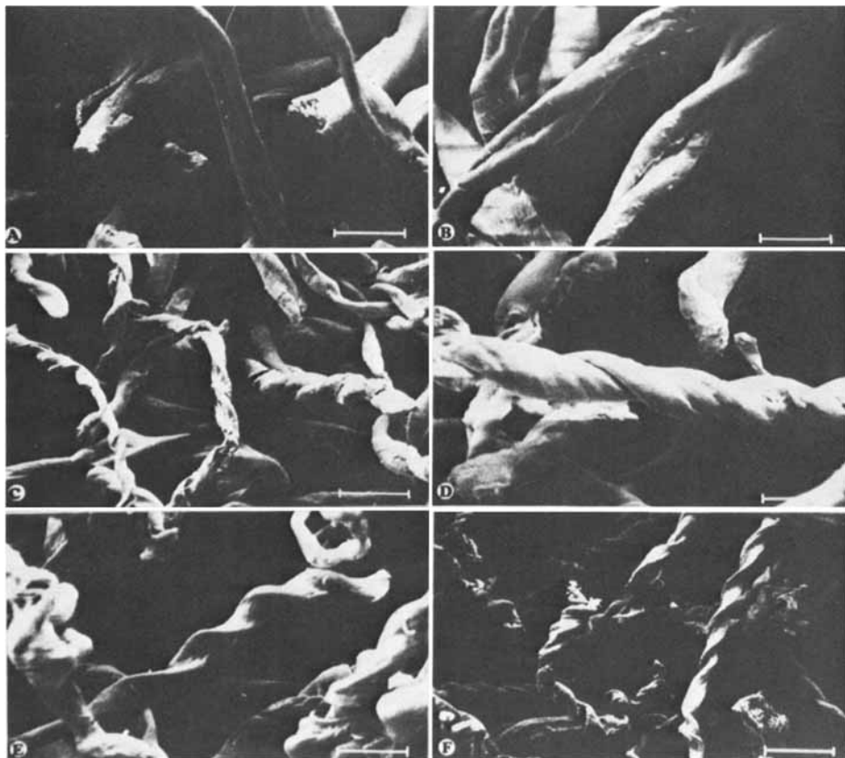
Fig. 9. Scanning electron micrographs of cellulose, scale 40\ \mu (A); and cellulose residues at 264^\circ\text{C} in air, scale 20\ \mu (B), at 284^\circ\text{C} in air, scale 40\ \mu (C), 298^\circ\text{C} in air, scale 20\ \mu (D), 326^\circ\text{C} in air, scale 20\ \mu (E), and 341^\circ\text{C} in nitrogen, scale 40\ \mu (F).
